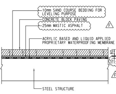
TYPICAL DETAILS FOR FOOTPATH PAVEMENT ON STEEL STRUCTURE
