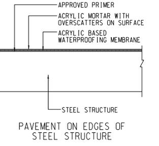
PAVEMENT ON EDGES OF STEEL STRUCTURE
