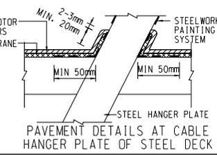
PAVEMENT DETAILS AT CABLE HANGER PLATE OF STEEL DECK
