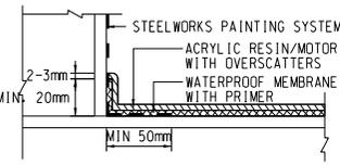
PAVEMENT DETAILS AT KERB OF OUTER STEEL DECK
