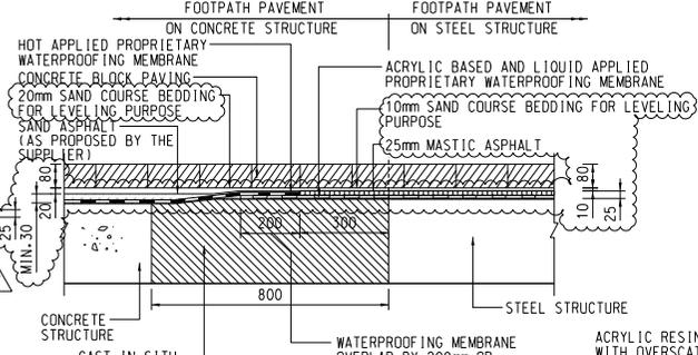
TRANSITION DETAILS BETWEEN FOOTPATH PAVEMENT ON CONCRETE STRUCTURE AND STEEL STRUCTURE
