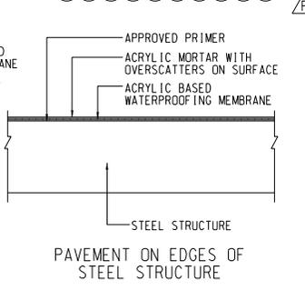
PAVEMENT ON EDGES OF STEEL STRUCTURE
