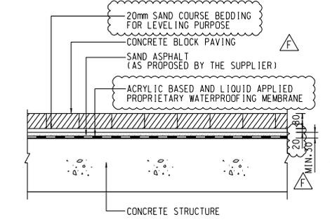
TYPICAL DETAILS FOR FOOTPATH PAVEMENT ON CONCRETE STRUCTURE
