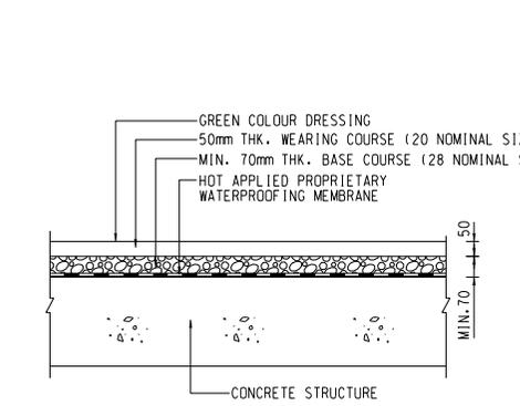
TYPICAL DETAILS OF CYCLE TRACK PAVEMENT ON CONCRETE STRUCTURE
