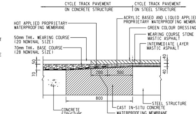
TRANSITION DETAILS BETWEEN CYCLE TRACK PAVEMENT ON CONCRETE STRUCTURE AND STEEL STRUCTURE
