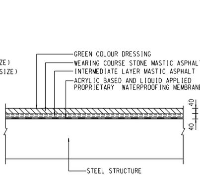
TYPICAL DETAILS OF CYCLE TRACK PAVEMENT ON STEEL STRUCTURE
