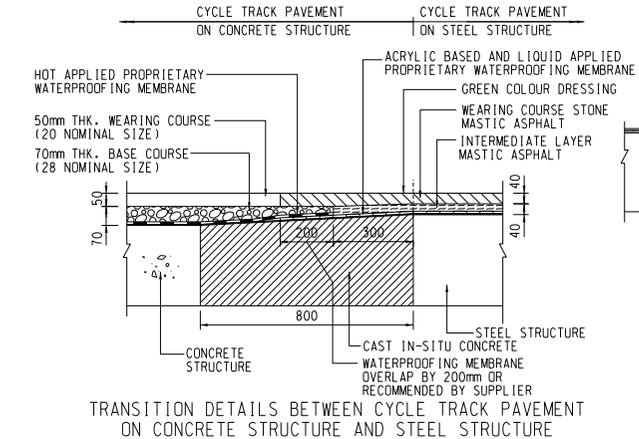
TRANSITION DETAILS BETWEEN CYCLE TRACK PAVEMENT ON CONCRETE STRUCTURE AND STEEL STRUCTURE
