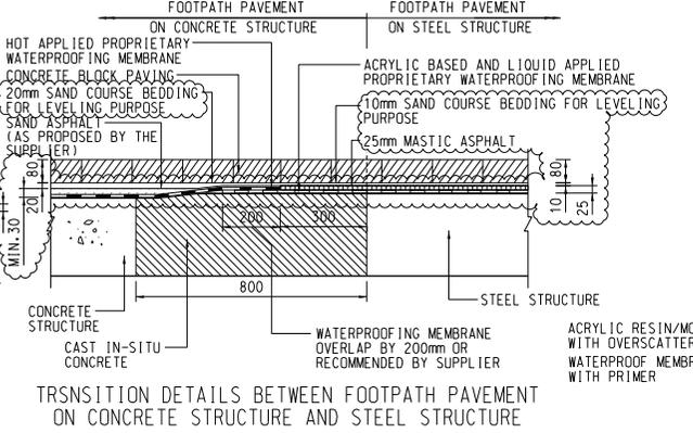
TRANSITION DETAILS BETWEEN FOOTPATH PAVEMENT ON CONCRETE STRUCTURE AND STEEL STRUCTURE
