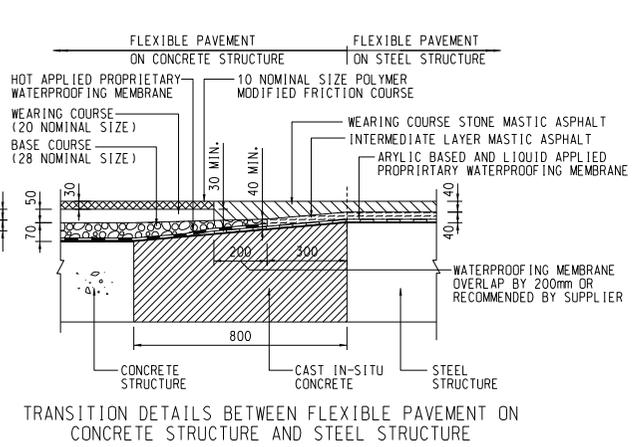
TRANSITION DETAILS BETWEEN FLEXIBLE PAVEMENT ON CONCRETE STRUCTURE AND STEEL STRUCTURE
